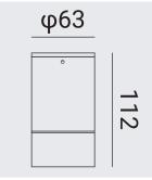
Modern black Outdoor waterproof mounted spot light in aluminum with COB LED / IP65 / 6w / 3000k warm white
