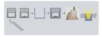
Stick the led strip with 3M tape to the flat bar. Put the aluminum flat bar to the led profile directly.
